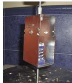
Sample subjected to load of 50 kg.
